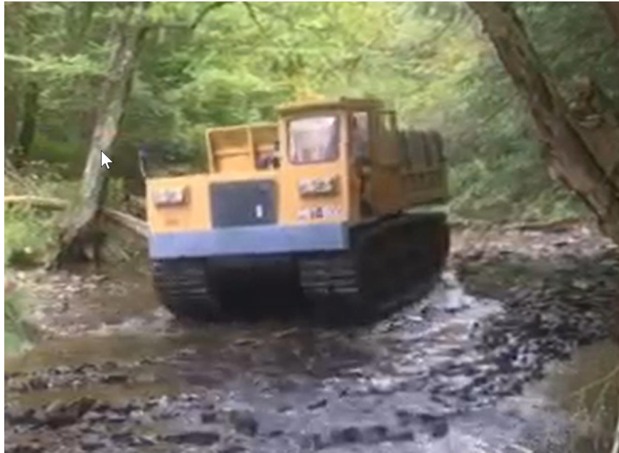
The wide tracks dispersed vehicle weight resulting in minimal impact.
